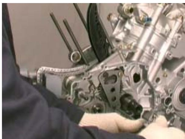
**3.9.3. REMOVING THE REAR TIMING UNIT**
