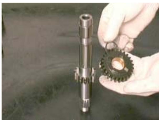
**4.2.2. REMOVING THE SECONDARY SHAFT**
